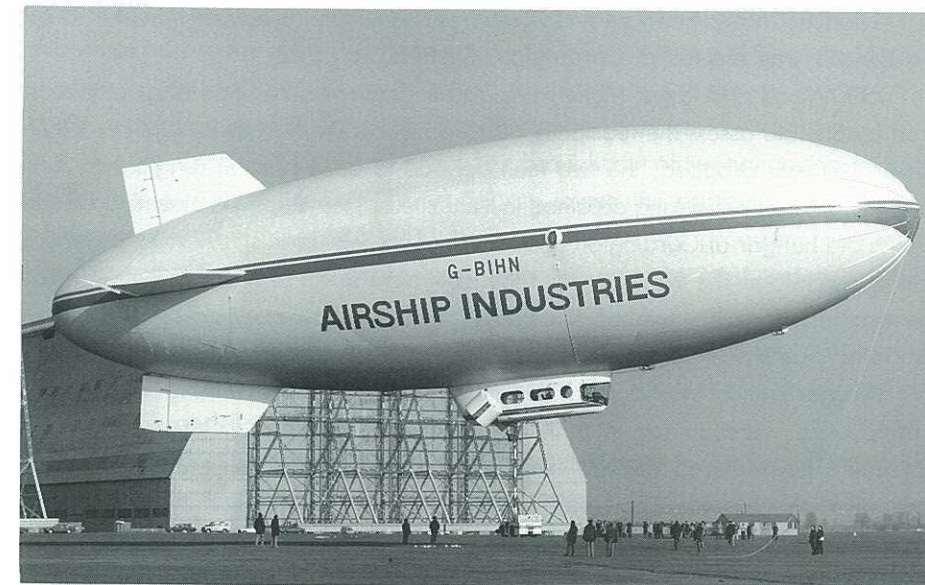
Launched in February 1979, at Cardington, England, the Skyship 500 is 164 feet long and 46 feet in diameter. When filled with 181,200 cubic feet of helium, she can carry up to eight passengers and a crew of two. Powered by two Porsche 930 engines, she has a top speed of nearly seventy miles per hour. The ship's propellers are mounted inside ducts for improved efficiency. They are also vectorable, that is, they can be turned downward as shown in the photo for added thrust during takeoffs and landings. Courtesy Airship Industries Ltd.
