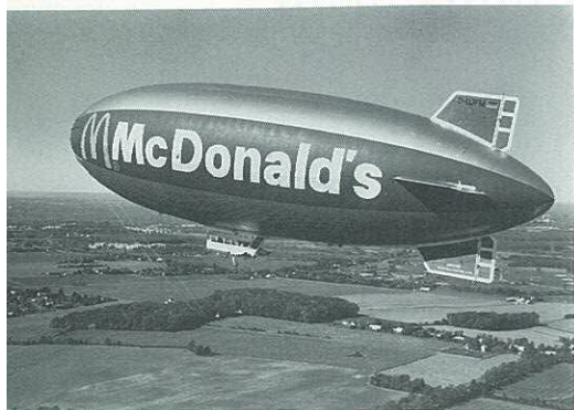
McBlimp was the second ship built by Theodor Wullenkemper in West Germany. His first blimp was launched by his Westdeutsche Luftwerbung in August 1972 and flew in Germany for several years before being sold to Japan. This was his first ship to reach the United States. McBlimp was 193 feet long and 54 feet in diameter, with 211,888 cubic feet of helium. She could carry up to eight people and featured a large computer-controlled night advertising sign similar to the ones on Goodyear blimps. McDonald's cancelled their lease after a number of franchises complained about paying for a blimp that was unlikely to ever visit more than a handful of the chain's restaurants. Since then, the ship has flown for Sea World and for Metropolitan Life. Courtesy McDonald's Corporation.
